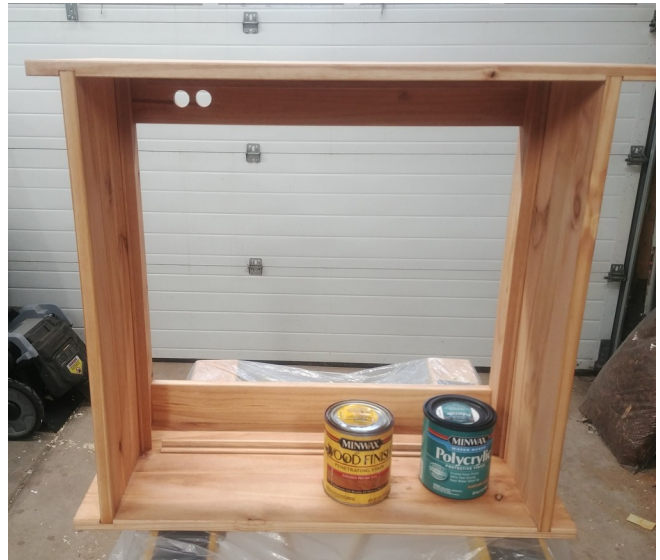
Figure 20: After sanding the whole frame with a 220-grit block (or similar), apply a coat of your stain of choice, followed by several protective layers such as polyurethane or polycrylic.
