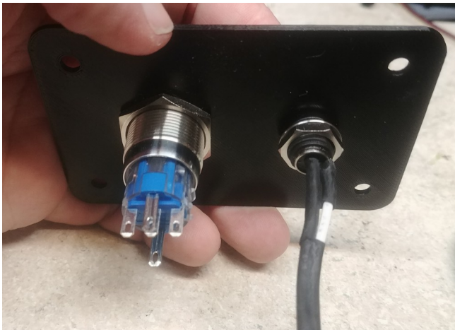
Figure 37: Install the 19mm halo switch and the barrel jack into the faceplate
