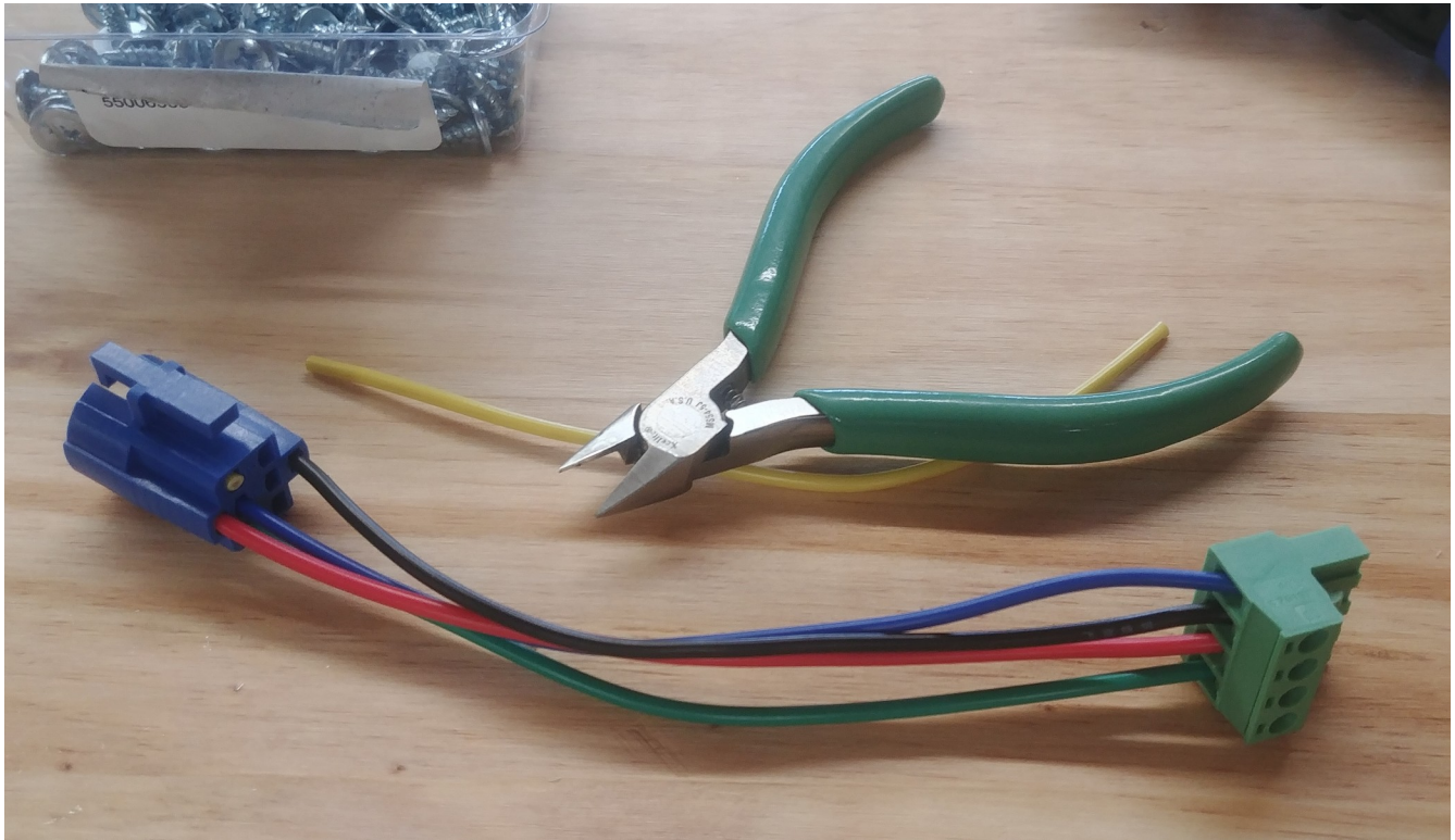
Figure 39: The wiring harness between the 19mm halo switch and the control board being assembled.
