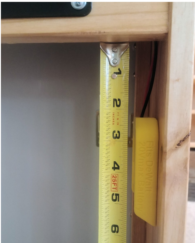
Figure 43: Leave yourself 2-3" above the battery connector
