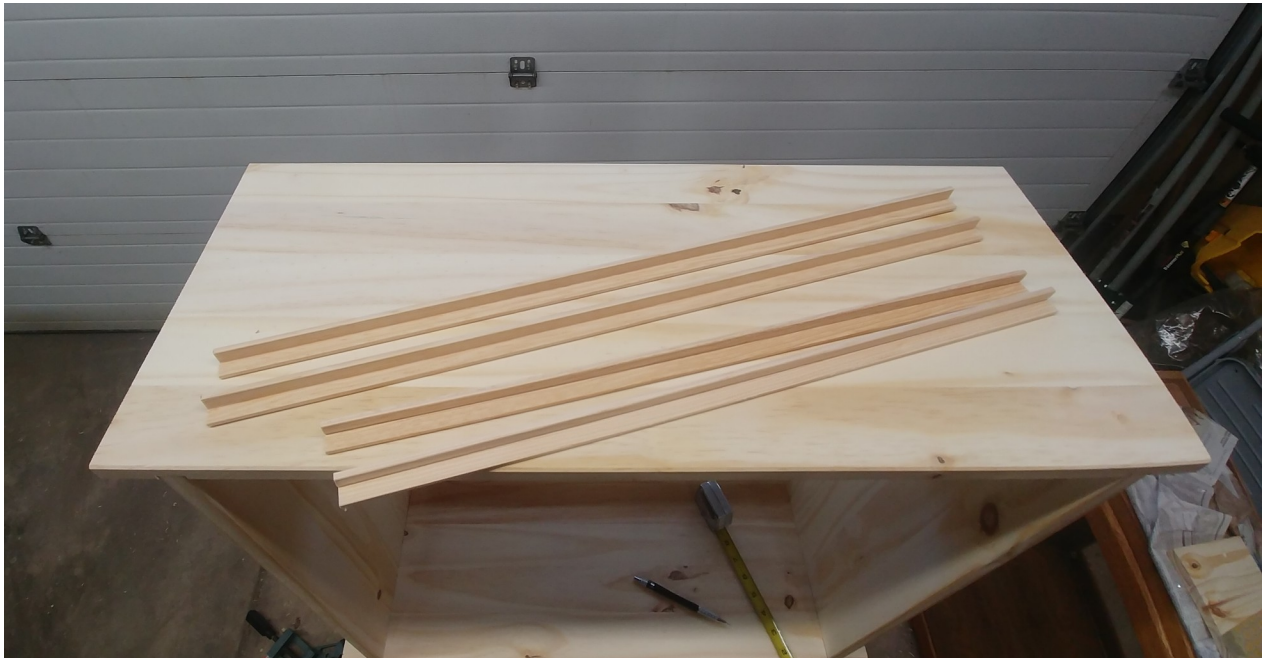
Figure 15: Cut two long (24-1/4") and two short (21") pieces of corner moulding in step 10.
