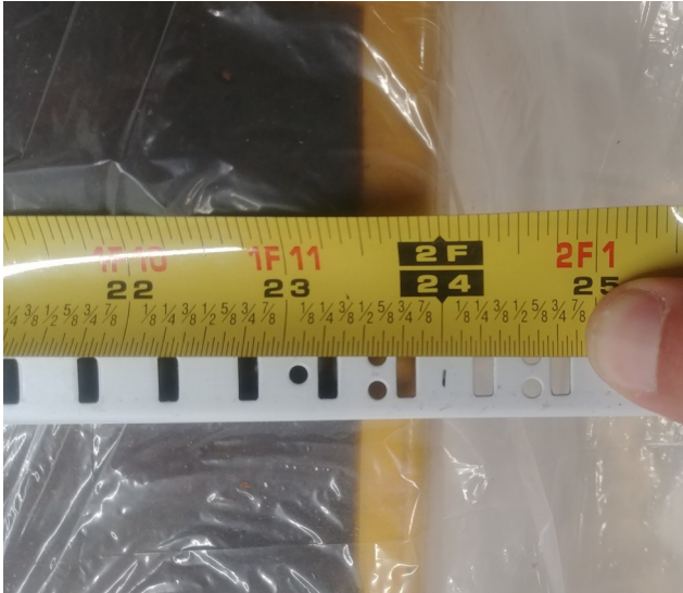
Figure 21: Cut a 24" section off each end of each shelf standard and throw away the center section. This makes sure we have a factory end on each section. The cut should fall between two of the double screw holes.
