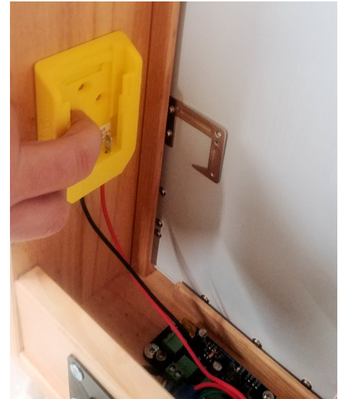
Figure 42: Positioning the battery connector on the inside wall, next to the switches and control board
