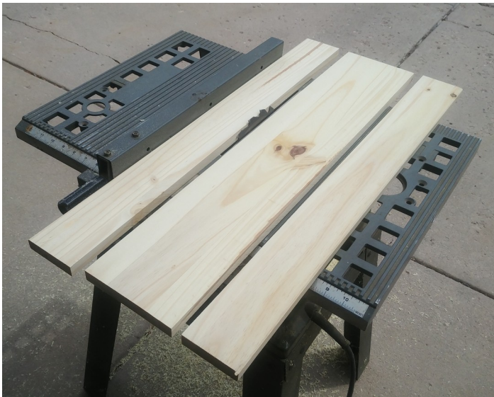
Figure 10: In step 6, use a table saw to cut a 3" piece off each side of the last shelf. These 3" pieces will be used in the back of the cabinet - the center piece is scrap.
