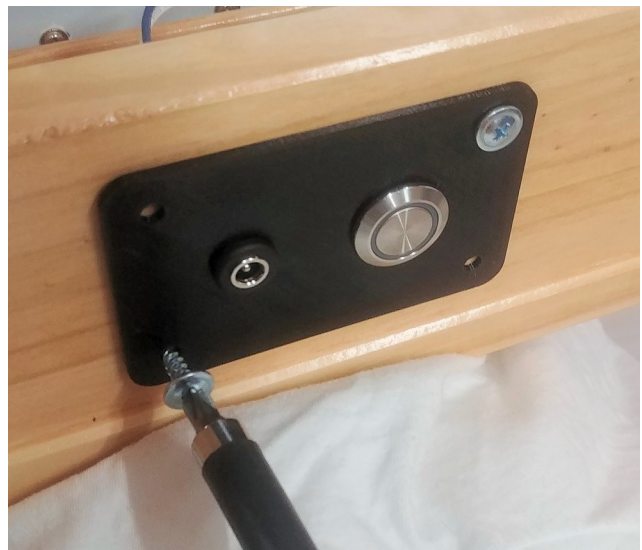
Figure 38: Install the faceplate over the two holes in the back of the case
