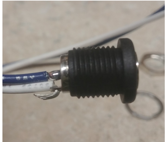
Figure 35: Solder each neatly to the jack, remembering which color went to the center (positive) and which went to the ring (negative).
