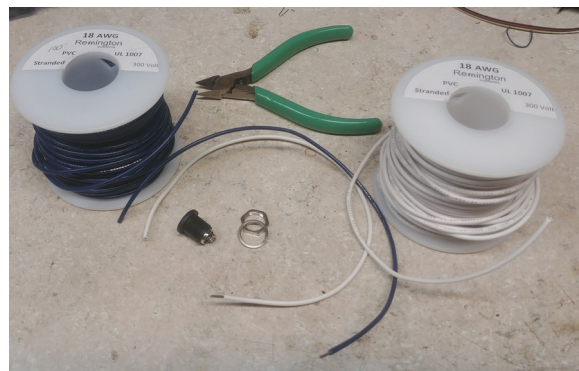
Figure 34: Cut two 10-inch 18AWG wires to attach to the barrel jack
