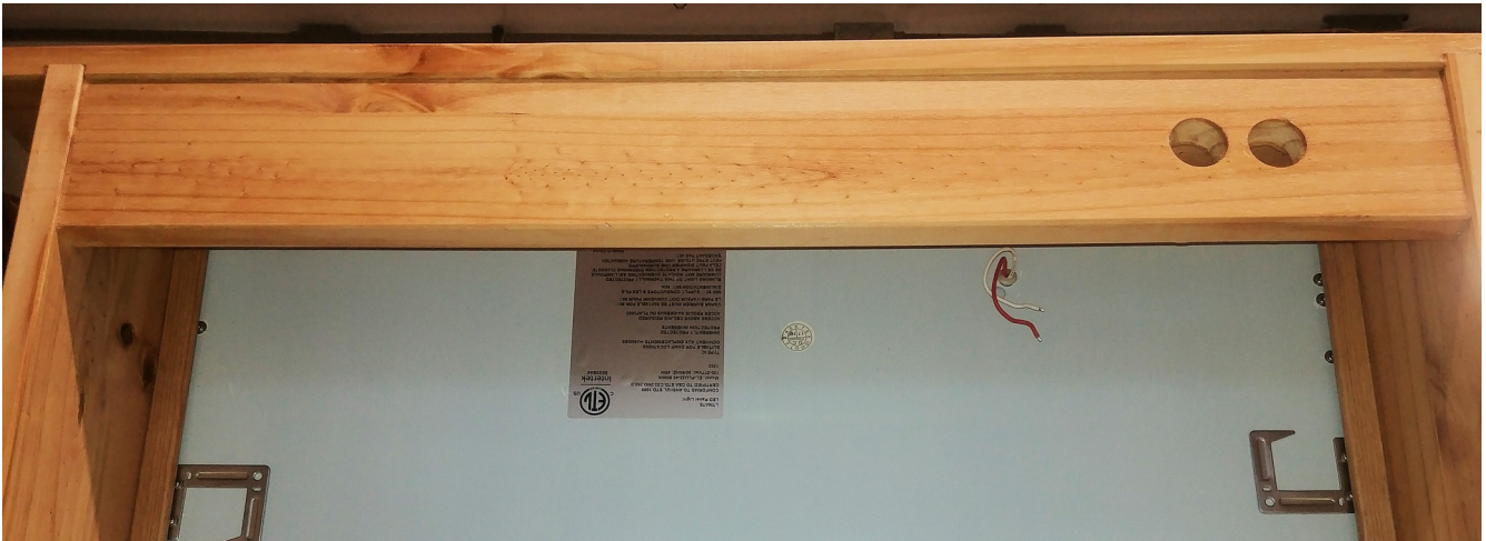
Figure 30: LED panel back in the cabinet, showing that the wires should be up near the holes
