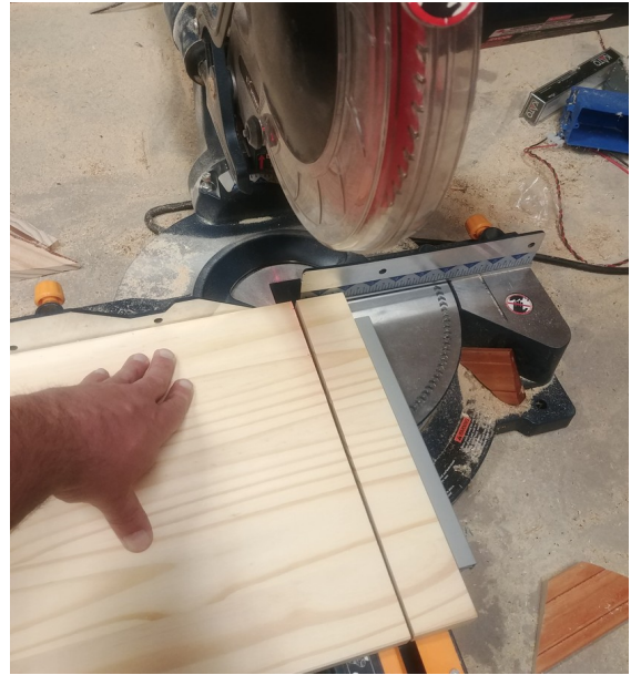
Figure 1- Cut the ends off the shelves leaving a little room – you don't want to saw through the parts of the grey plastic ends that are inserted.
