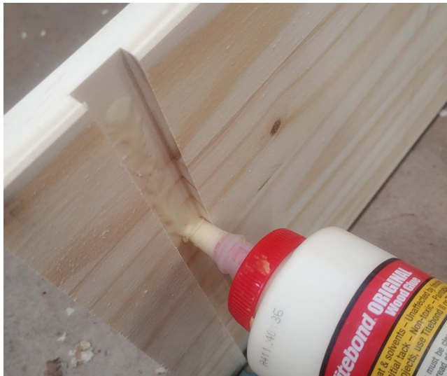
Figure 6: Gluing the sides to the top and bottom is critical for strength, but don't use too much or it will squirt out.
