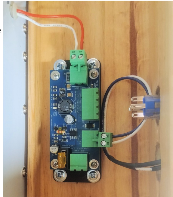
Figure 40: Connect the barrel jack wires to the PCB. In this picture, negative (white) is on top, positive (blue) is on bottom.
