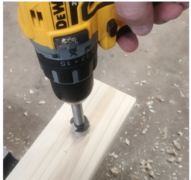
Figure 11: In step 7, use a nice sharp Forstner bit to drill two holes (one for the switch, one for the 24V power jack) in the top rear brace.
