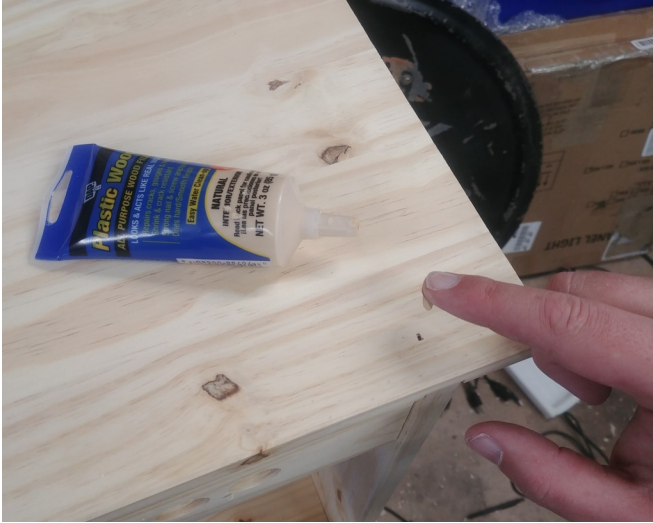
Figure 19: Fill any nail holes or other obvious imperfections with stainable wood putty, wait until dry, and sand down flat
