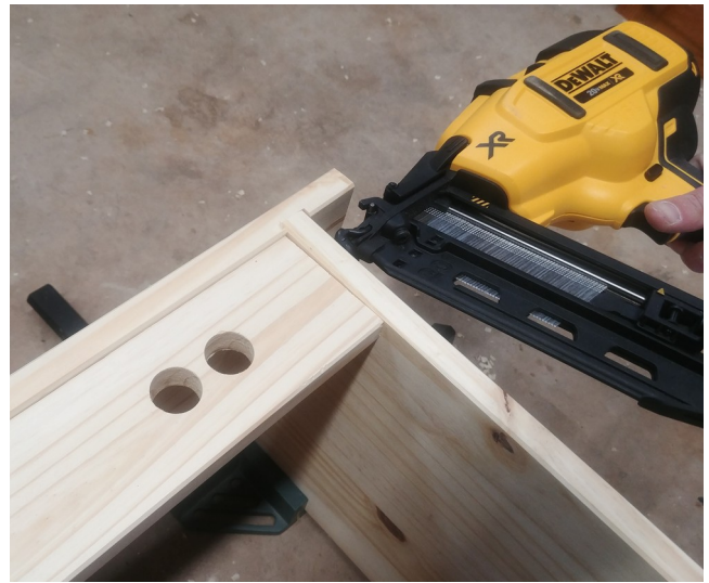
Figure 13: Use finishing nails driven in from the sides to secure the rear top and bottom brace boards
