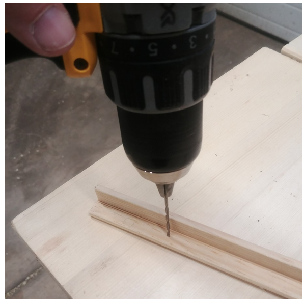
Figure 16: Drill three holes through one side of each piece of corner moulding. These will hold nails that will secure it to the frame.
