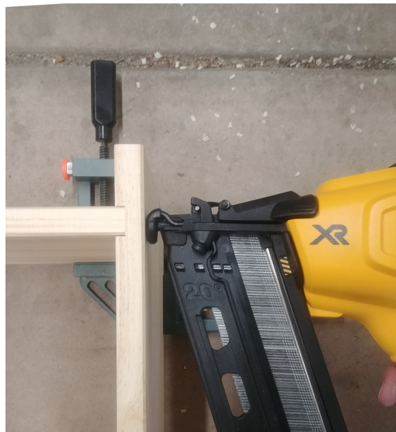
Figure 9: Carefully driving 16ga finishing nails into the top helps hold everything square and makes it extra strong
