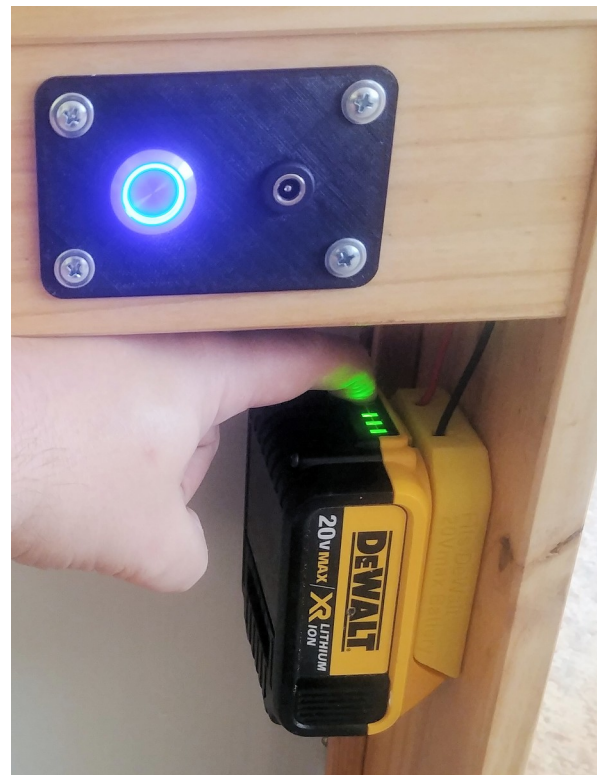
Figure 44: This is why you've left a few inches above the battery - you want to be able to reach in and hit the battery gauge button to see how much power you have left
