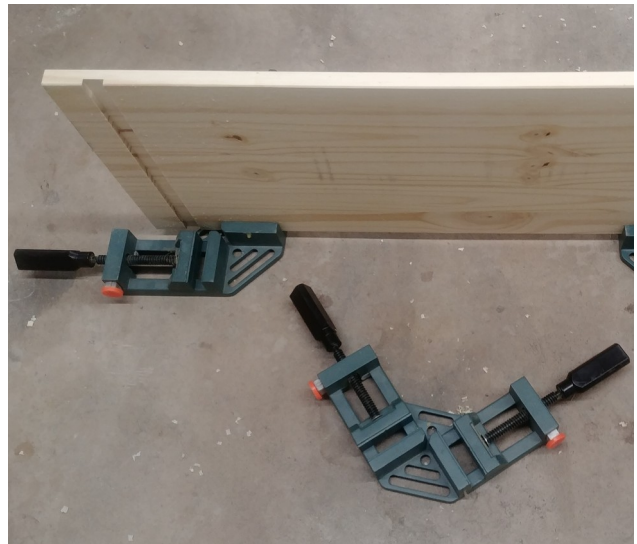
Figure 7: Setting up one of the end boards with some 90 degree clamps from Harbor Freight.
