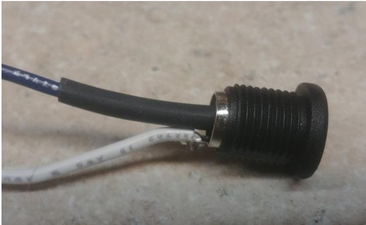
Figure 36: Once soldered, apply heat shrink insulation to guard against shorts
