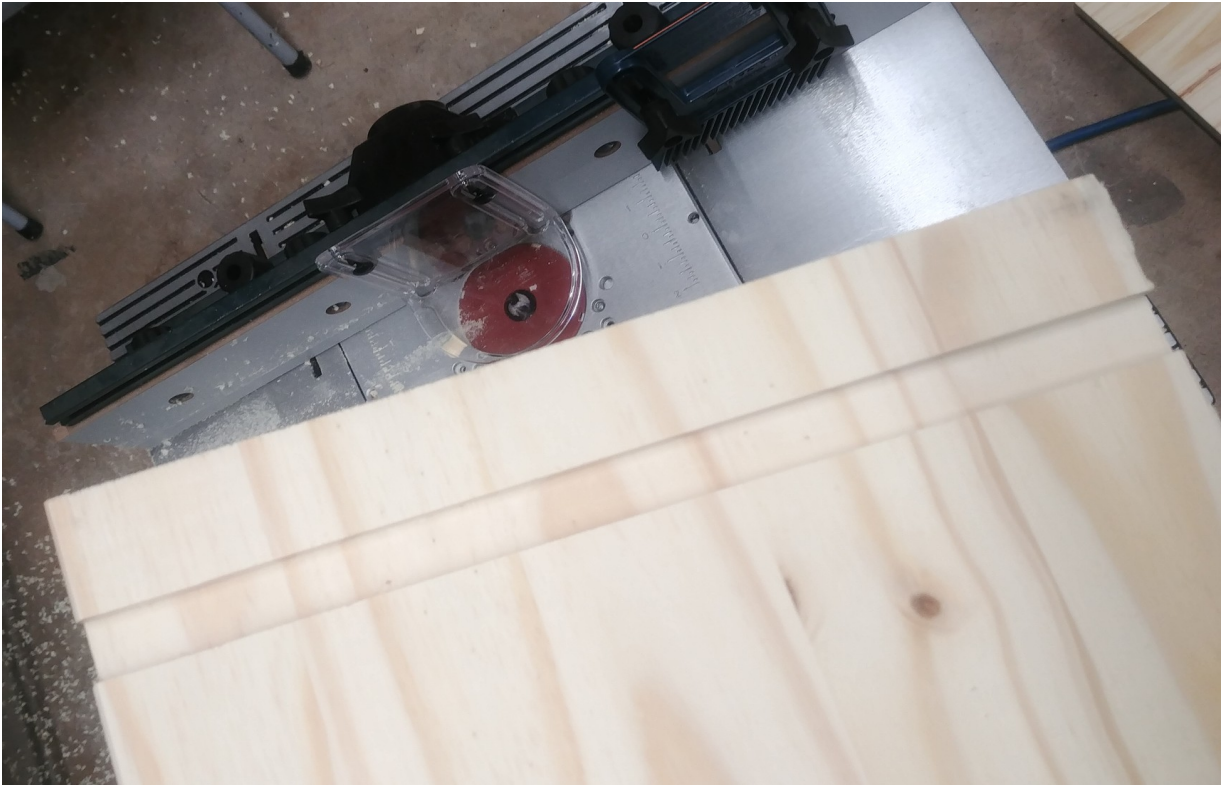
Figure 4 - This is what the finished cut should look like at the end of Step 3. These dado channels should be on the top of the bottom board and the bottom of the top board, and will help hold the sides in place.
