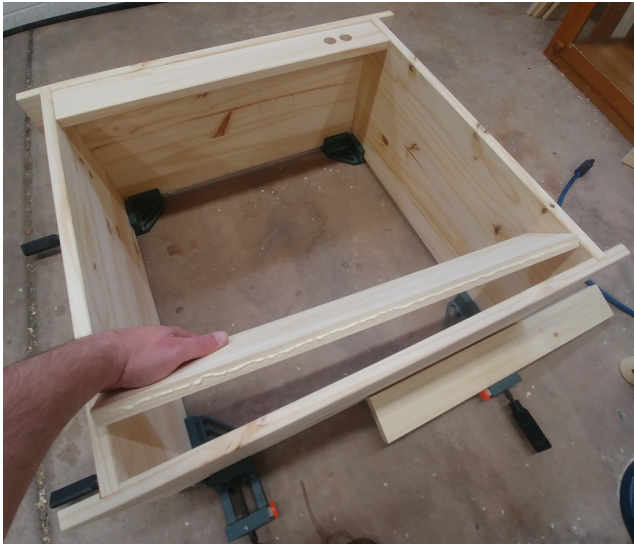
Figure 12: Install the rear top and bottom brace boards using a thin bead of glue on the long edge only.
