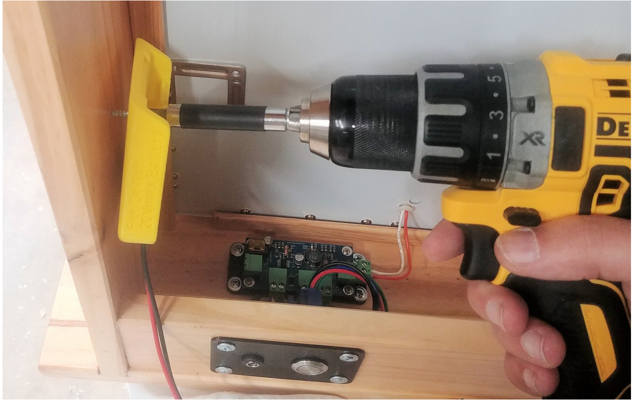
Figure 45: Be sure to drill pilot holes before driving screws! Mount the battery connector to the wall using #8 x 3/4" flat head screws.
