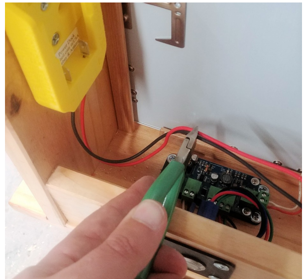
Figure 46: Trimming battery connector leads
