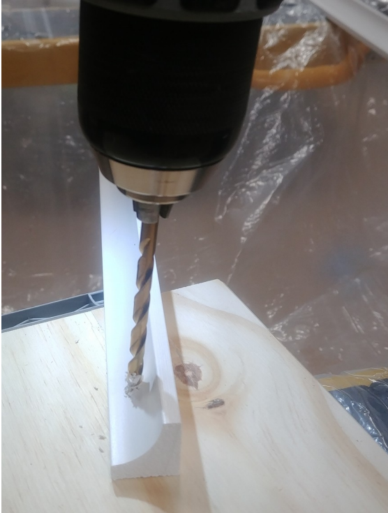
Figure 25: Drill three holes straight down through the PVC moulding on the side that will mate with the inside top/bottom of the cabinet
